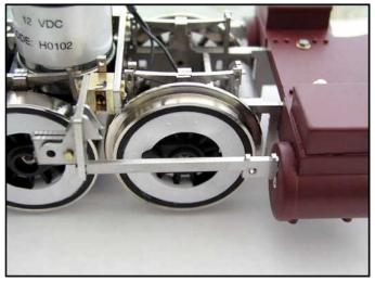
Here's a closer view of the crosshead guide support bracket packer.
