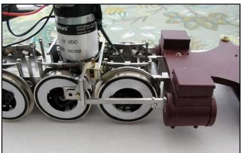
Beginning with the image to the left the next series of photos by Andy Bernat, as he assembles the chassis to working order: Note 7.4mm packer made from brass to space the crosshead guide supports to the correct location.
