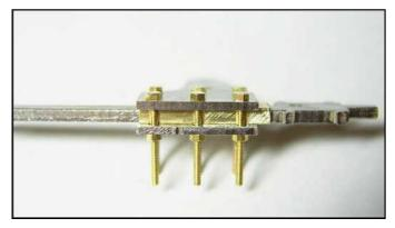
The brass SHS between the inner and outer crosshead plates is to be different from the standard MC2002 instructions above, as we are not using 3.2mm x 3.2mm Plastruct SHS. Instead the guide is 2mm thick, and 3.4mm deep. Use K&S brass tube  $3/16" \times 3/32"$  RHS. Grind out slots into the sides of the RHS allowing the bolts to pass across the RHS as seen to the left. This will hold the RHS from sliding out.
