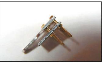
It would be a good idea to file out the holes in the side rods a little to remove the sharp edges inside the holes. These sharp edges may cut away at the crank pins!
