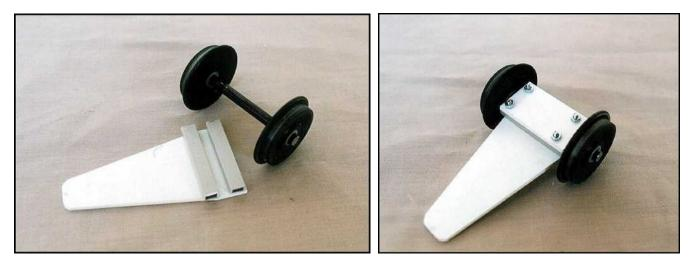
The pivot for the pilot truck will be a vertical 4.6mm x 4.6mm ABS Plastruct SHS mounted vertically on the front spacer of your chassis. Just bolt the SHS to the center front of the forward spacer. Then insert a bolt through the truck and screw into the hollow centre of the SHS.
