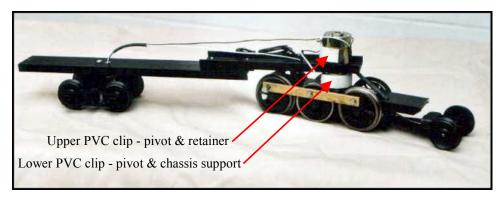
**Note:** Barry also initially used a PVC pipe clip between the chassis and frame as a bearing pad, but we changed it as part of the spring rigging design in chapter 2. The tender deck assembly from chapter 2 also needs to be sandwiched between the two frame channels, with the deck flat down on top of the rear channel.
