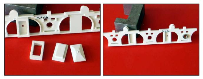
Now, build the two beams that will be placed between the side frames. Mine are 10mm x 17mmand x 62mm long. Make them as long as you need to fit our axles into the bearings. I use LGB axles and have copied the width of an LGB truck. You can make the beams solid or hollow, as you wish. Mine are hollow and filled with lead.
