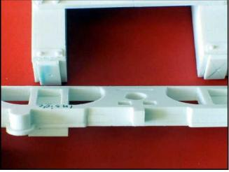
Glue one (only one!) side frame to the beams. Be sure everything is square. The remaining side frame will be screwed from the outside to the beams later. Prepare holes for the screws like shown above.
