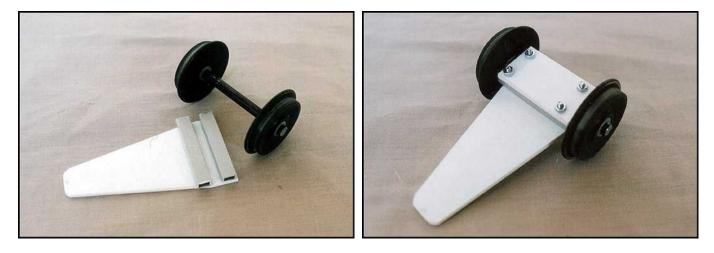
The pivot for the pilot truck will be a vertical 4.6mm x 4.6mm ABS Plastruct SHS mounted vertically on the front spacer of your DIY chassis. Just bolt the SHS to the center front of the forward spacer. Then insert a bolt through the truck and screw into the hollow centre of the SHS.
