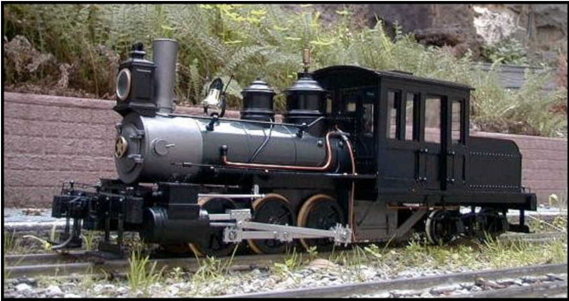
It was quite common in the 1870s for the boiler bands to be made from Russia Iron material, matching the boiler jacket. It also happens to be damn stylish! or
