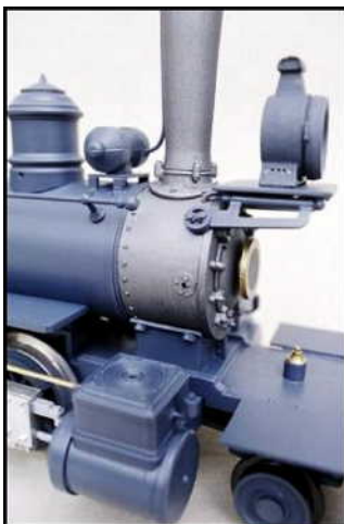
Rivets along rear end of smoke box.
