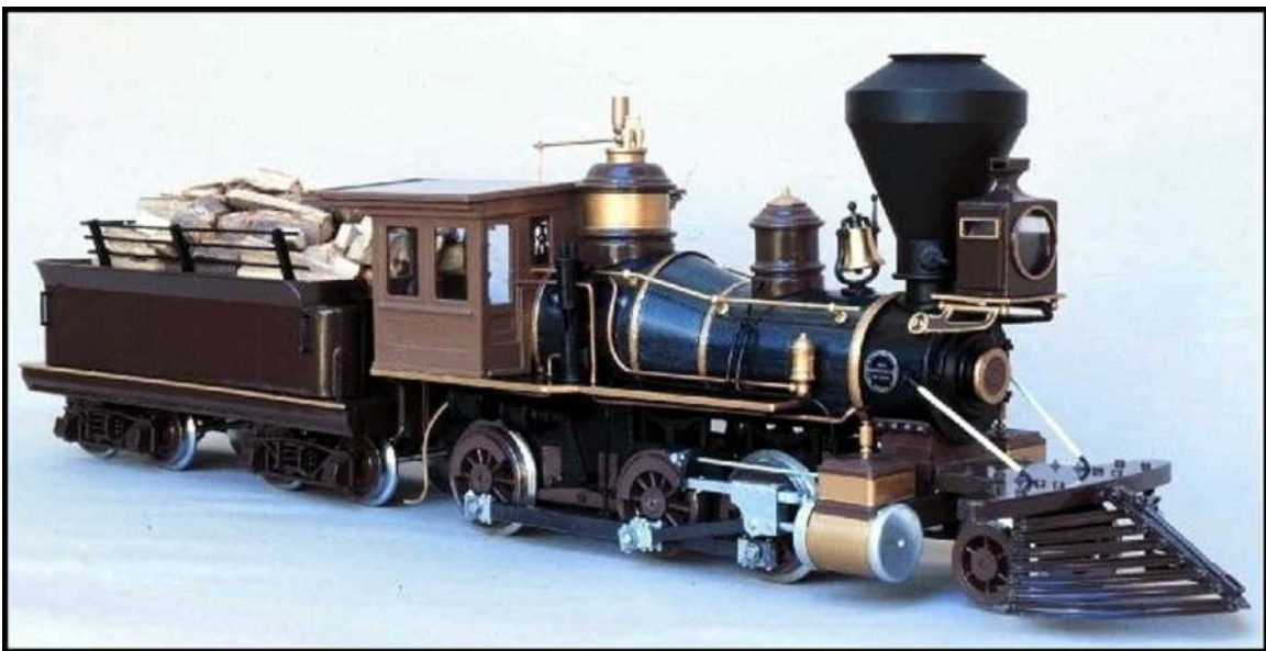
...Paint the boiler bands a brass color! The color scheme of this loco is also demonstrates my attempt at doing a 'Lake' color scheme to a 1870s Baldwin 2-6-0. Lake is a very dark brown. The boilers in both of these models were painted using automotive spray cans.
