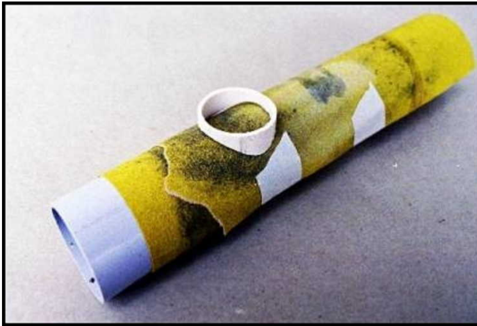
The 51mm PVC pipe clad in sand paper and my dome base being sanded to the right profile by grinding the thing back & forth over the pipe!!
