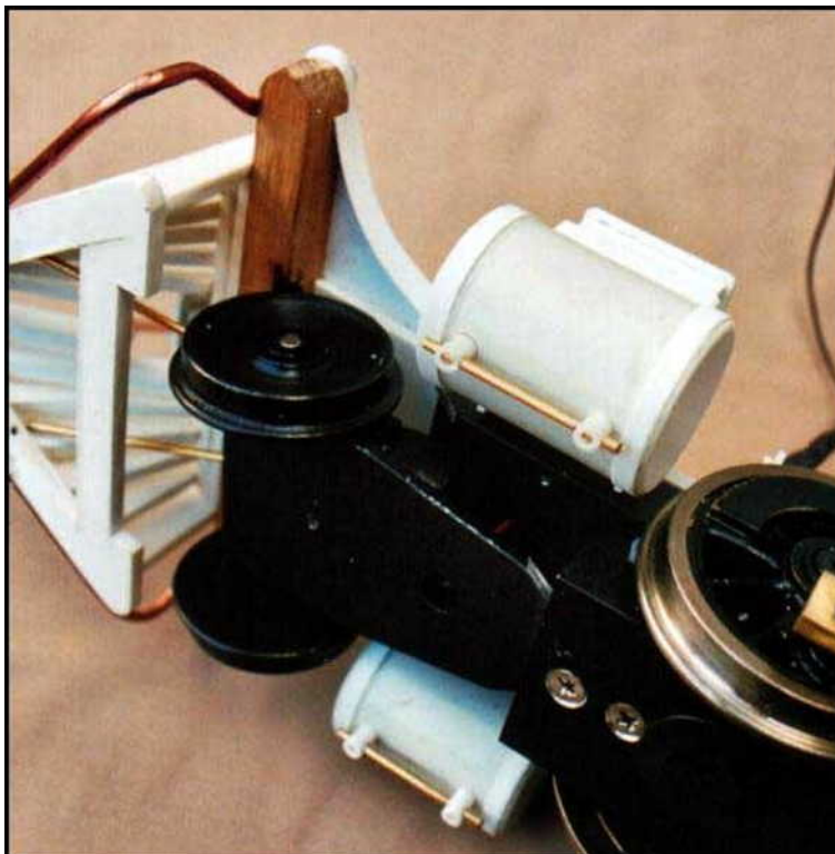
The cylinder drain cocks shown installed at the base line of both cylinders.
