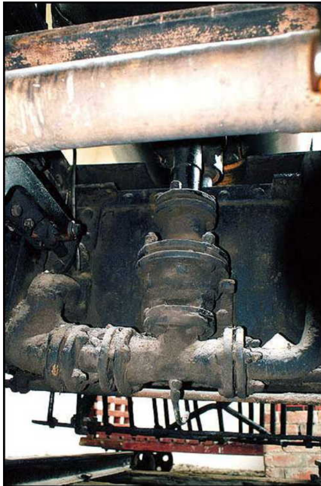
Leave it to intrepid Dave to get under the bogie! Here's a shot of the steam pipe arrangement (interior bogie chassis).
