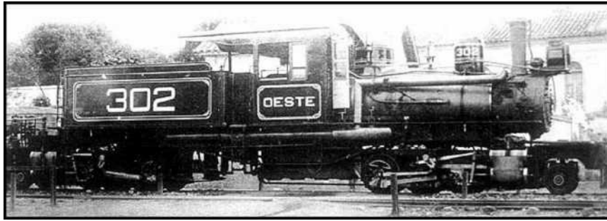
Here's a Kitson-Meyer built out of a Shay!
