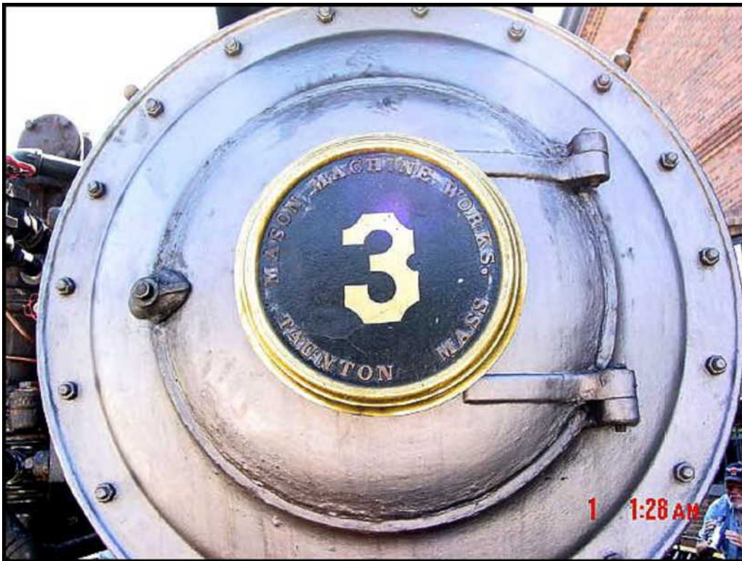
The Smokebox door, Original Mason style down to the plate!
