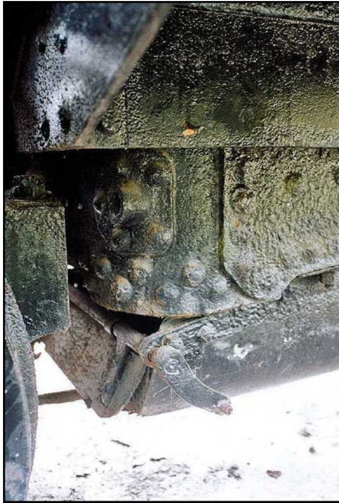
A view of the front end of the firebox. Note the forward dampers, like we made on our Mason models.
