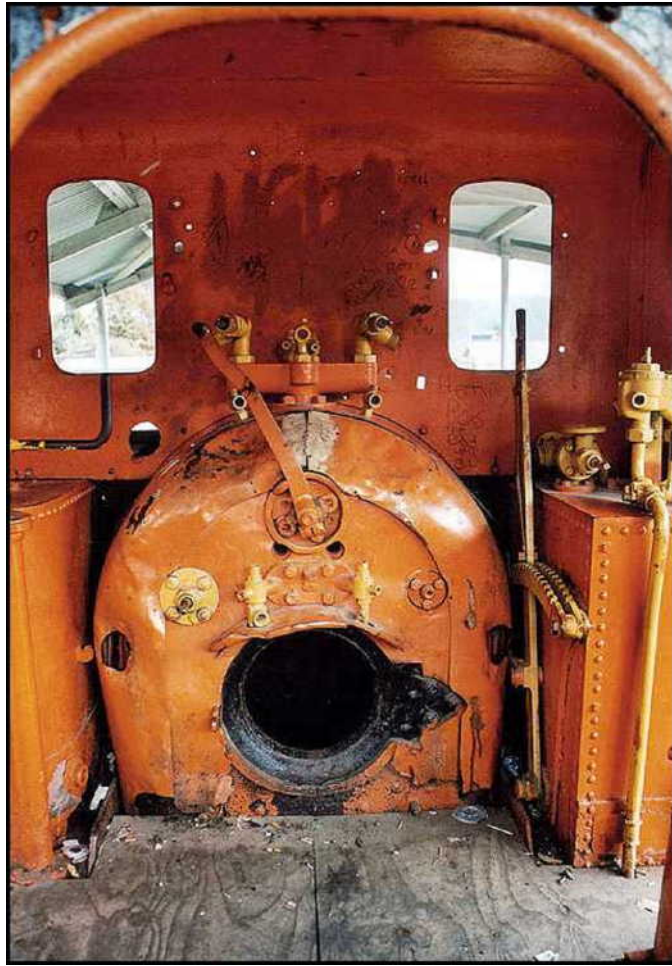
A view of the dilapidated backhead.
