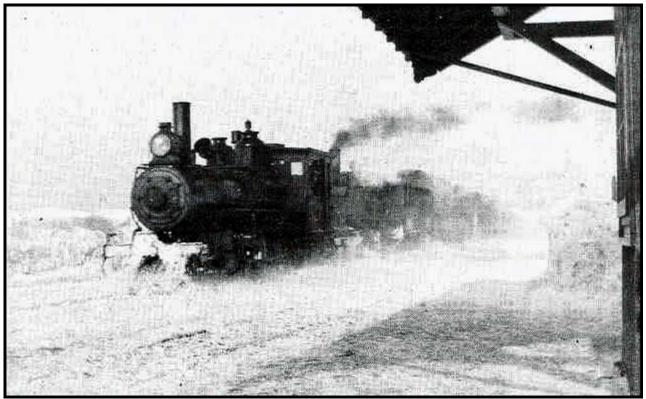
Figure 40 - After having finally been successful in clearing the Winthrop Loop for traffic, here we see two Mason Bogies working in tandem to keep things moving around the Loop. (BSRA)
