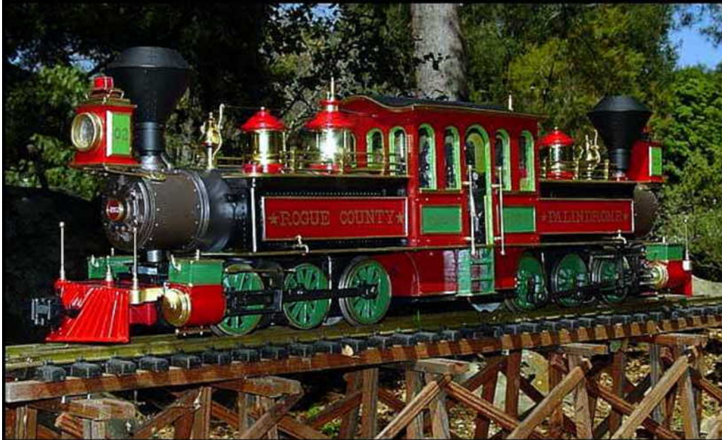
As a source of inspiration, MC2001 Master, Chris Walas, eager to get building a Mason-like machine before the class started, built this superb rendition of what a Mason Built narrow gauge Double Fairlie would have looked like. The loco, named 'Palindrome' is inspired by Mason's 'Janus' and is built to the Narrow Gauge scale of 1:20.3. Well done Chris!
