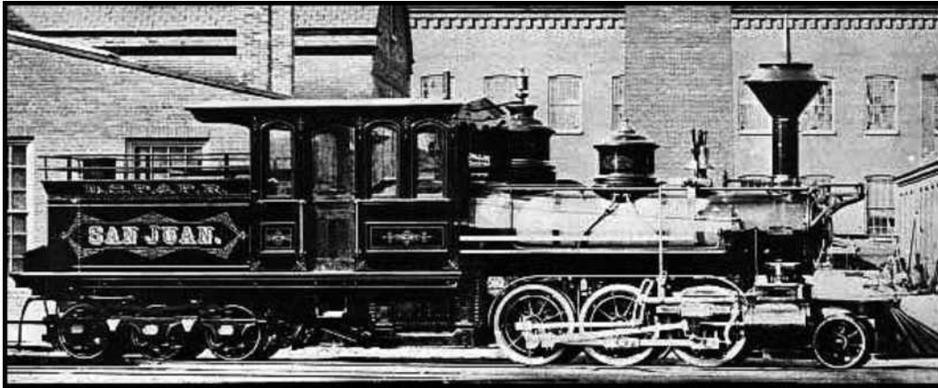
Builder's Photo of the first 2-6-6T Mason Bogie delivered to the South Park, DSP&P #4 'San Juan' of 1878.
