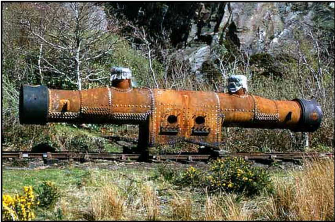
The disused boiler of an Ffestiniog Double Fairlie 0-4-4-0. Note the double firebox serving the two independent boilers.
