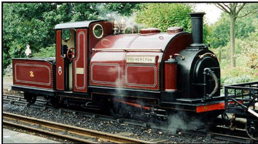
A typical George England 0-4-0 of 1864, restored at the Ffestiniog. 'Palmerston'.
