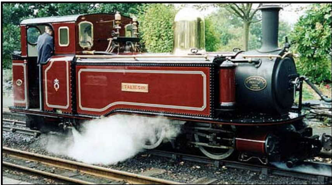
The 'Taliesin', a replica Single Fairlie, now at work on the Ffestiniog Railway.
