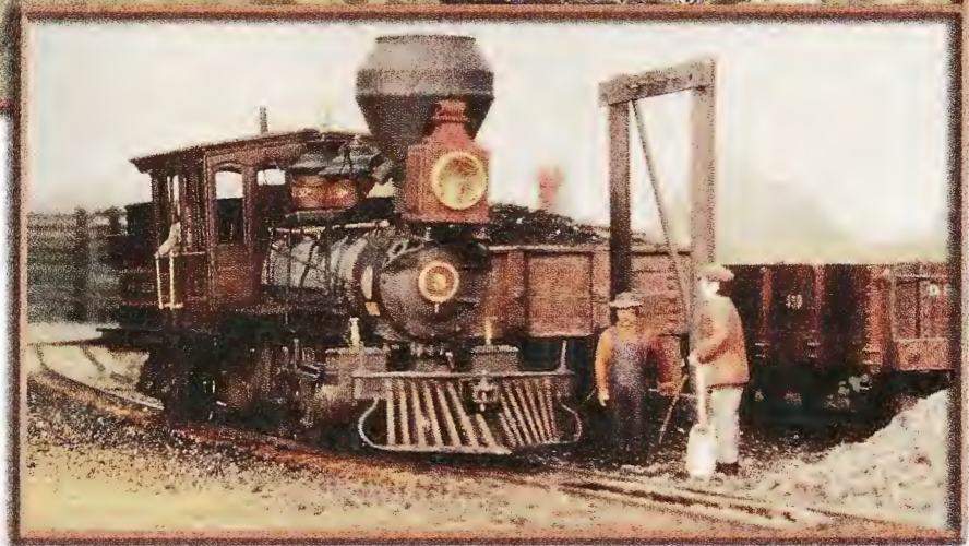
Right: Number 3, ORO CITY, originally arrived on the South Park as an 0-6-6T, but was later fitted with a pony truck while still retaining its Nesmith stack and arched cab windows.
