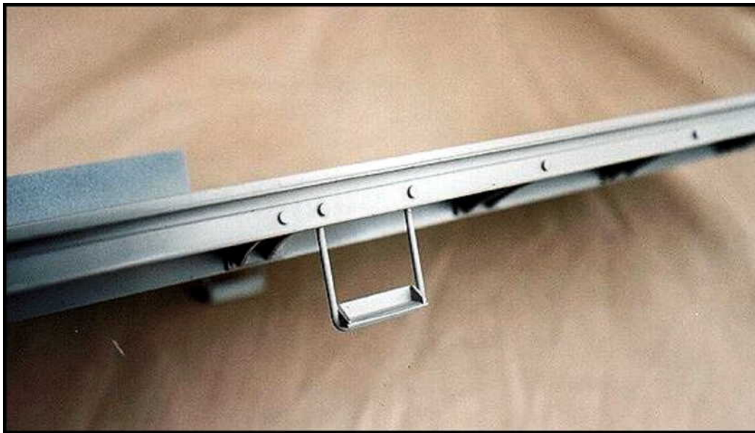
Cab step as seen from outside the deck. Note how the new step stirrup aligns with the two special rivets added back in Chapter 2.
