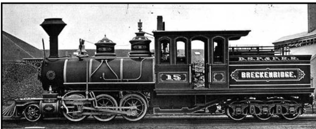
The 'Breckenridge' posing for a photo at the Mason plant, again the loco has been equipped with a 'Fontaine stack' for the purpose of the photo. The loco was actually delivered to the South Park with a 'Nesmith Stack'.
