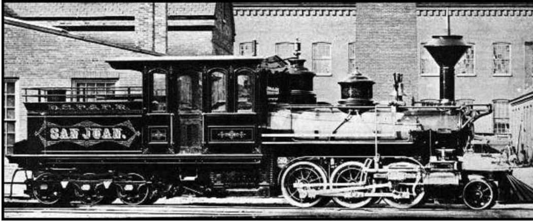
The beautiful 'San Juan', photographed at the Mason plant with a small diamond stack called a 'Fontaine Stack'. The spec sheets show this loco actually delivered to the South Park with no stack actually fitted. Mason would never let possible ugliness get in the way of a good photo if his locos!
