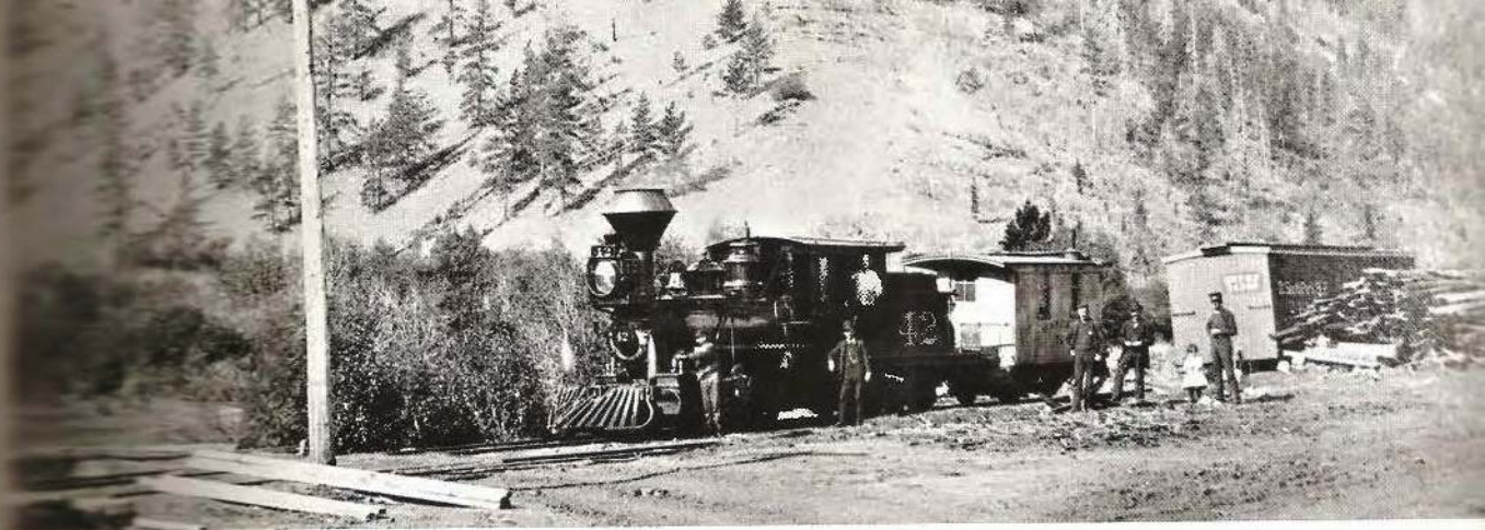
Figure 4: Jackson photographer's special train at Webster in 1886. The locomotive is Mason Bogie 2-6-6T Number 42 with Waycar Number
