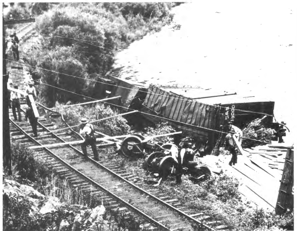
Photo 3. Another view of the car in Photo 2. The lateral roofwalks next to the cupola are similar to those on 306 in Photo 1. A rod brace is visible off the corner of the cupola. There is no roofwalk along the length of the cupola.
