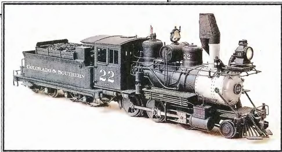
C&S #21 was rebuilt from an inexpensive Bachmann On30 model using a number of brass castings from PSC, Backshop, PIA, Coronado Scale Models, and Kemtron.
