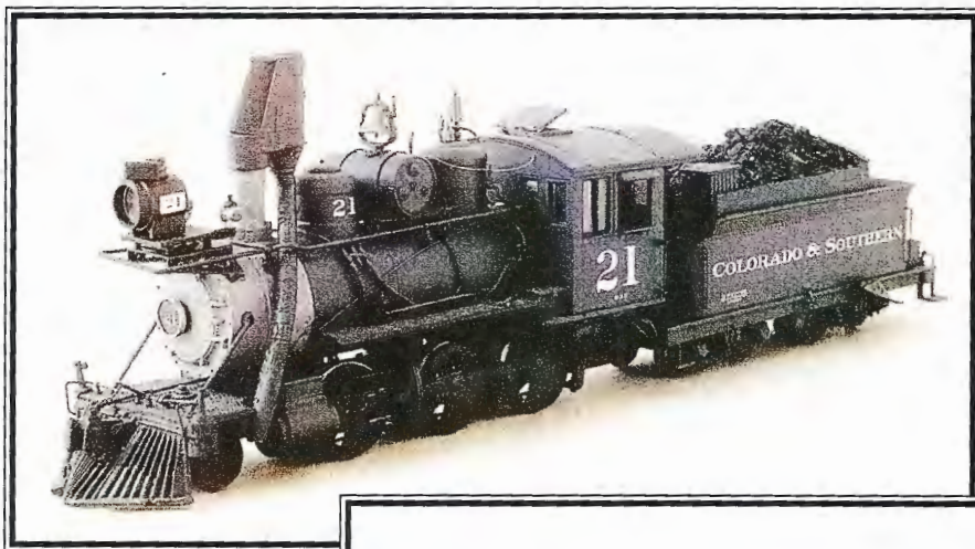
C&S #21 was rebuilt from an inexpensive Bachmann On30 model using a number of brass castings from PSC, Backshop, PIA, Coronado Scale Models, and Kemtron.
