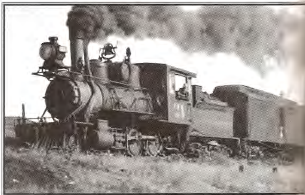
Below: Some have reported that C&S #21 never received one of the Ridgway patented smokestacks. This Otto Perry photo proves otherwise. She is shown smoking out of Denver on Train 70 in July 1918.
